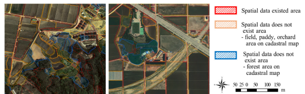
Fig. 5. Characteristics of the spatial data not exist areas based on the current land use classification system and the corresponding Cadastral Map
