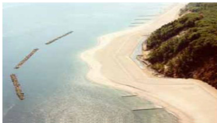
(c) Detached breakwater
