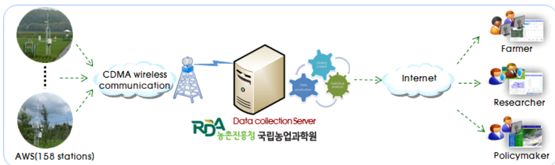
Fig. 5. Flowchart of agrometeorological information service in Rural Development Administration (RDA) of Korea.
